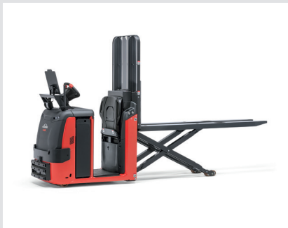
Scissor lift for back-friendly picking
